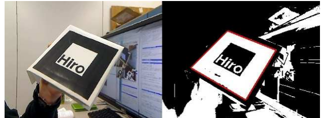
Fig.4 Monochrome for Marker tracking
